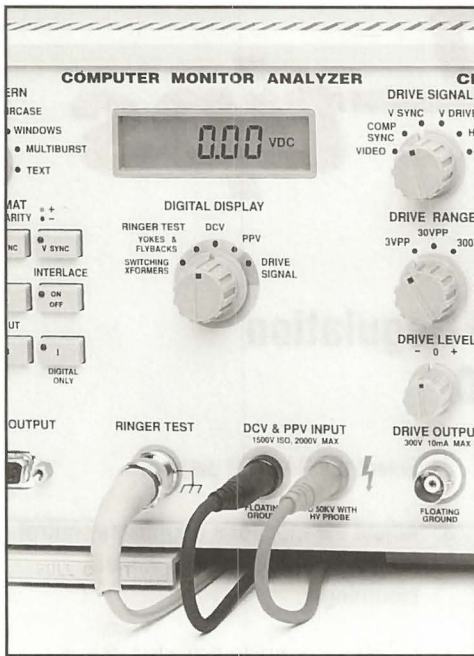
Fig. 2: Use the Digital Display functions to measure the DCV and PPV at the horizontal output transistor.
