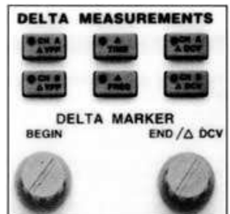
Fig. 8: The Delta functions allow you to measure just a portion of the waveform.
