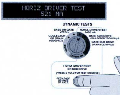
Fig. 3: The Horiz. Driver Test is a dynamic test that measures the output drive current capability of the horizontal driver stage.
