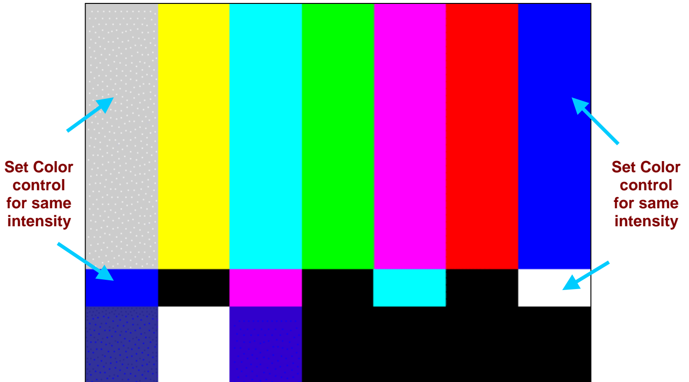
Fig 5: View the SMPTE bar pattern blue through a blue filter. Adjust the Color control to make the top and bottom outside bars the same intensity.
