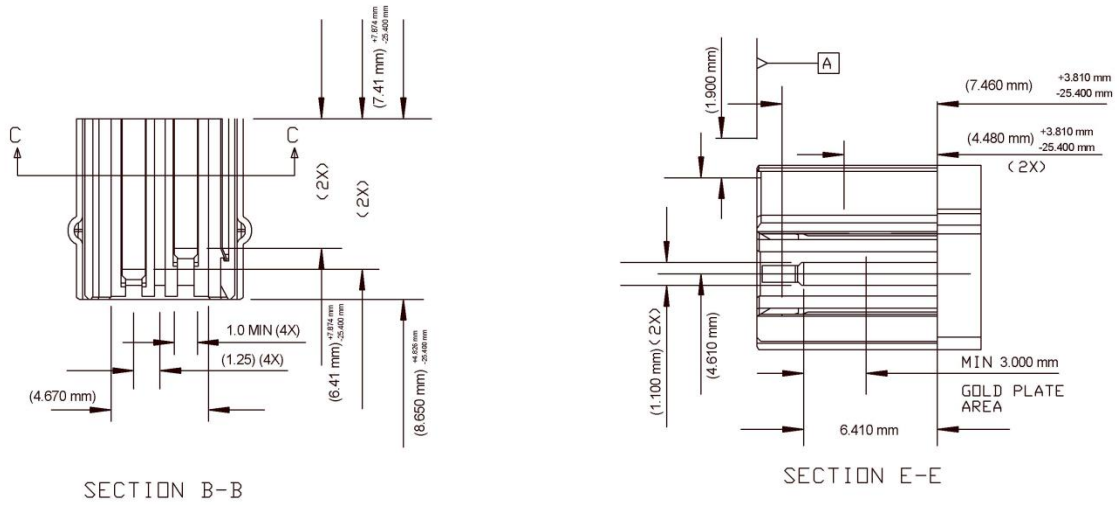
Figure 3-14 USB 2.0 PD Standard-B Plug Interface Dimensions
