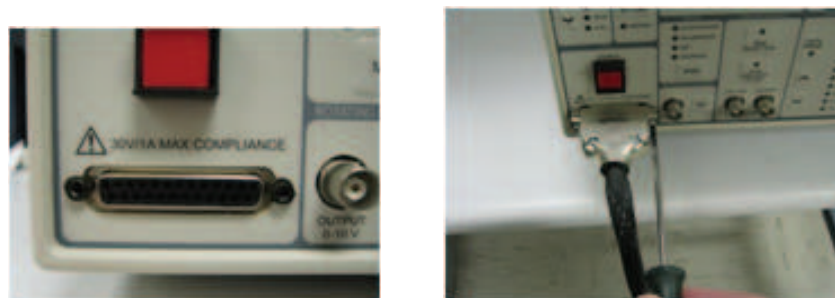
Figure 5: Front panel umbilical connector on EC301. Securing the umbilical cable to the EC301.
