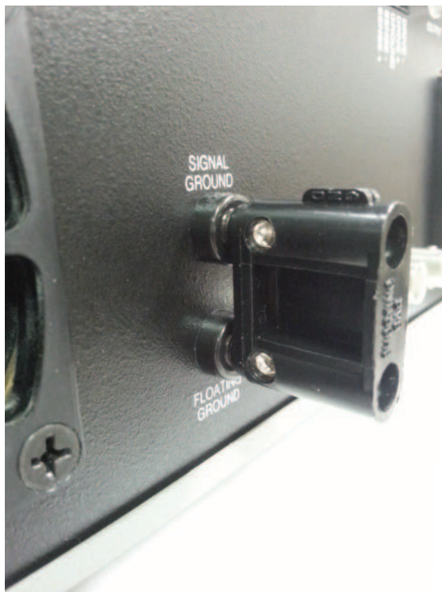
Figure 13: EC301 grounding bar (installed).
