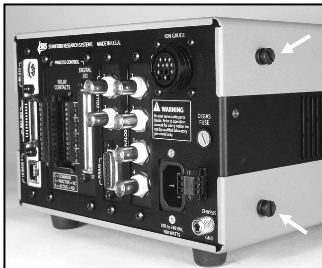
Figure L-3. Mounting pins in place.
