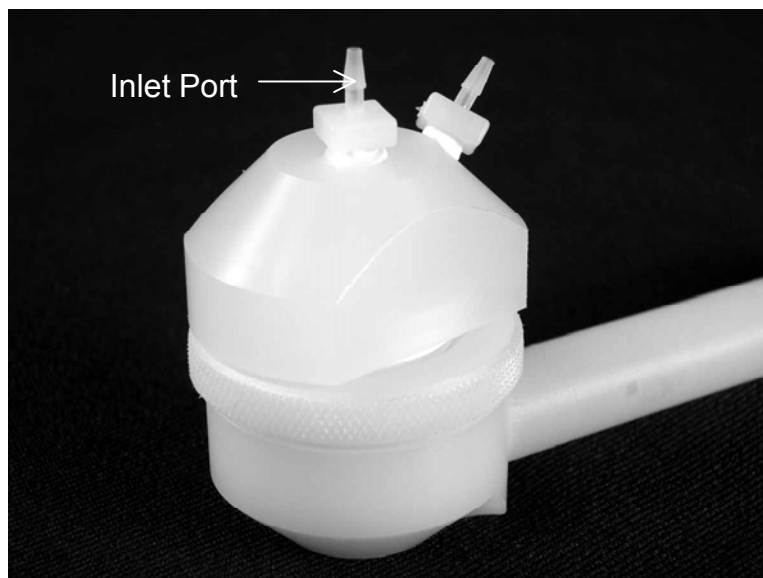
Figure 12. The axial flow cell adapter mounted on a crystal holder.
