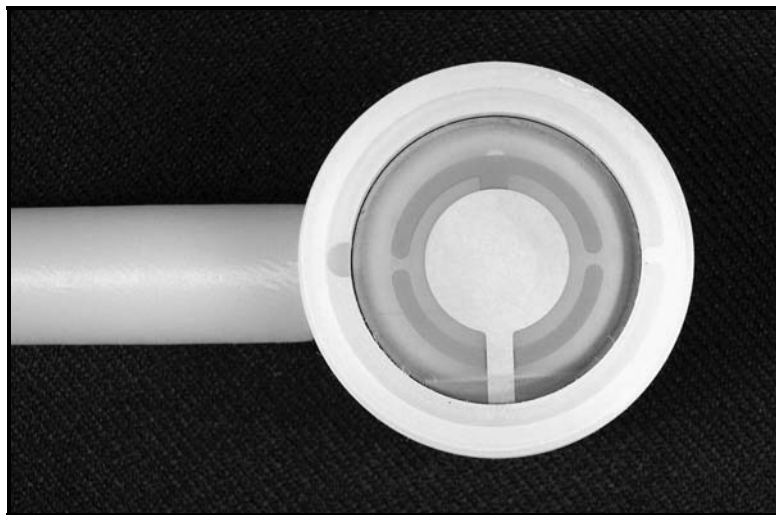
Figure 7. Crystal in place with correct electrode orientation.
