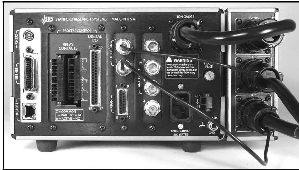
Figure L-6. An IGC100 with an O100IG option installed and two Ion gauges connected to its back panel. Decide up front which gauge you want to connect to the IG1 port and which one to the IG2 port.
