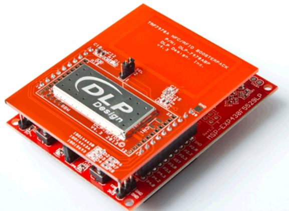
Figure 37. F5529 LaunchPad With DLP-7970ABP NFC BoosterPack
