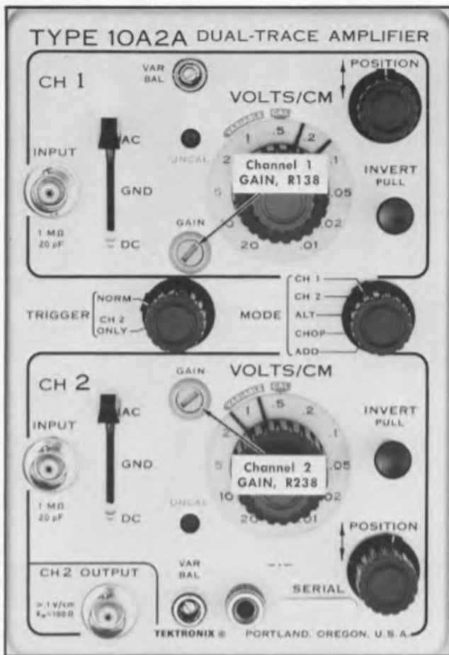
Fig. 6-7. Location of channel 1 GAIN control, R138 and channel 2 GAIN control, R238.
