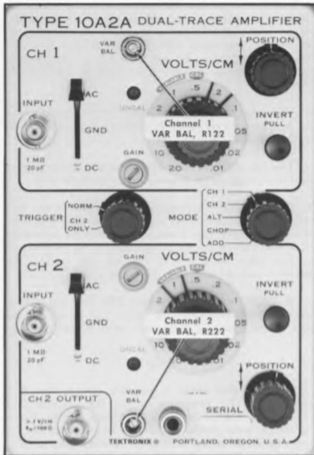
Fig. 6-4. Location of channel 1 VAR BAL control, R122 and channel 2 VAR BAL control, R222.
