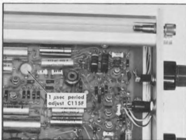
Fig. 4-10. Location of 1 microsecond period capacitor C115F.
