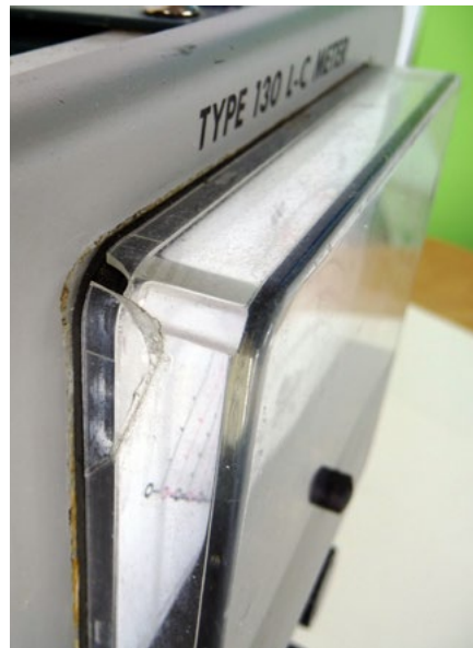
The front panel glass was cracked along one edge. There was also grime and dirt inside and outside the case.
