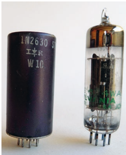
A 1N2630 (left) was used instead of the original 6X4 (right) as the rectifier. Due to its larger diameter and weight, it came loose from the socket in transit, damaging one of the 6U8s.
