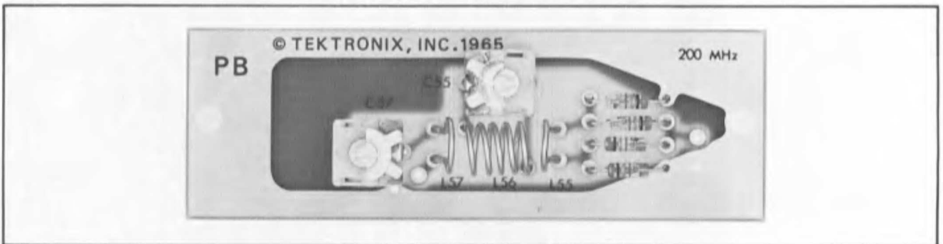
Fig. 4-6. 200 MHz (5 ns) etched-wiring board.
