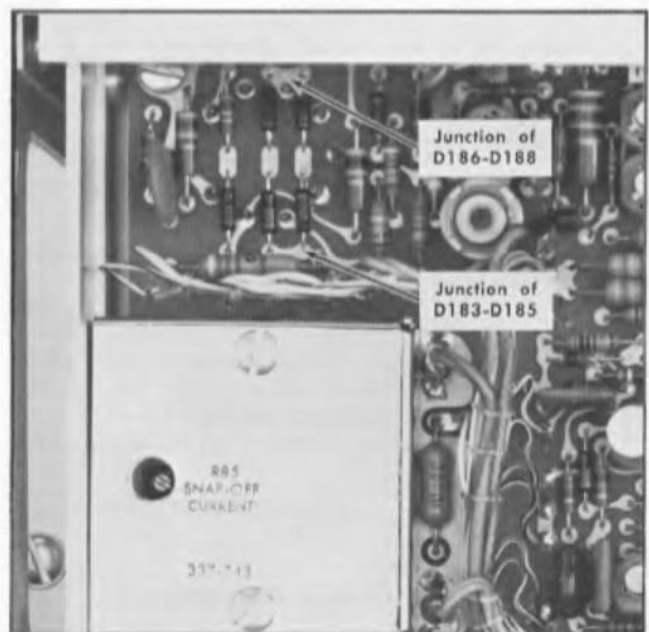
Fig. 5-42. Left side of Type 1S1 showing test points for checking dc vertical output voltage.
