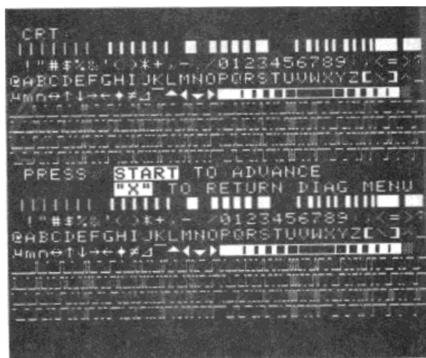
Figure 5-7. 318 CRT test parallel acquisition character fonts.
