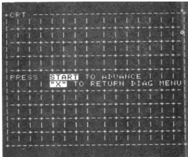
Figure 5-5. 318 CRT test cross-hatch pattern.
