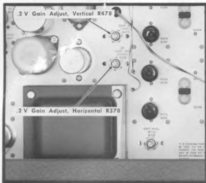
Fig. 6-12. Location of .2 V Vertical and Horizontal gain adjustments.
