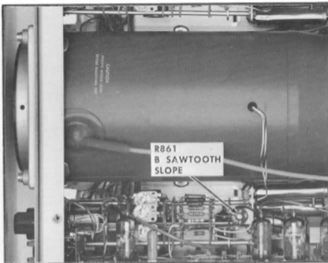
Fig. 6-35. Adjustment location for B sweep sawtooth slope.
