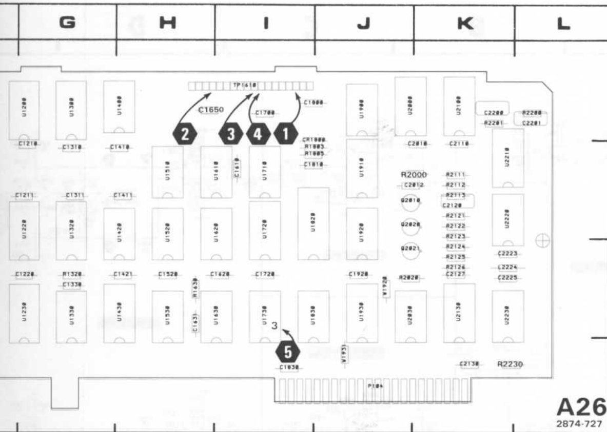
Control Logic circuit board assembly.
