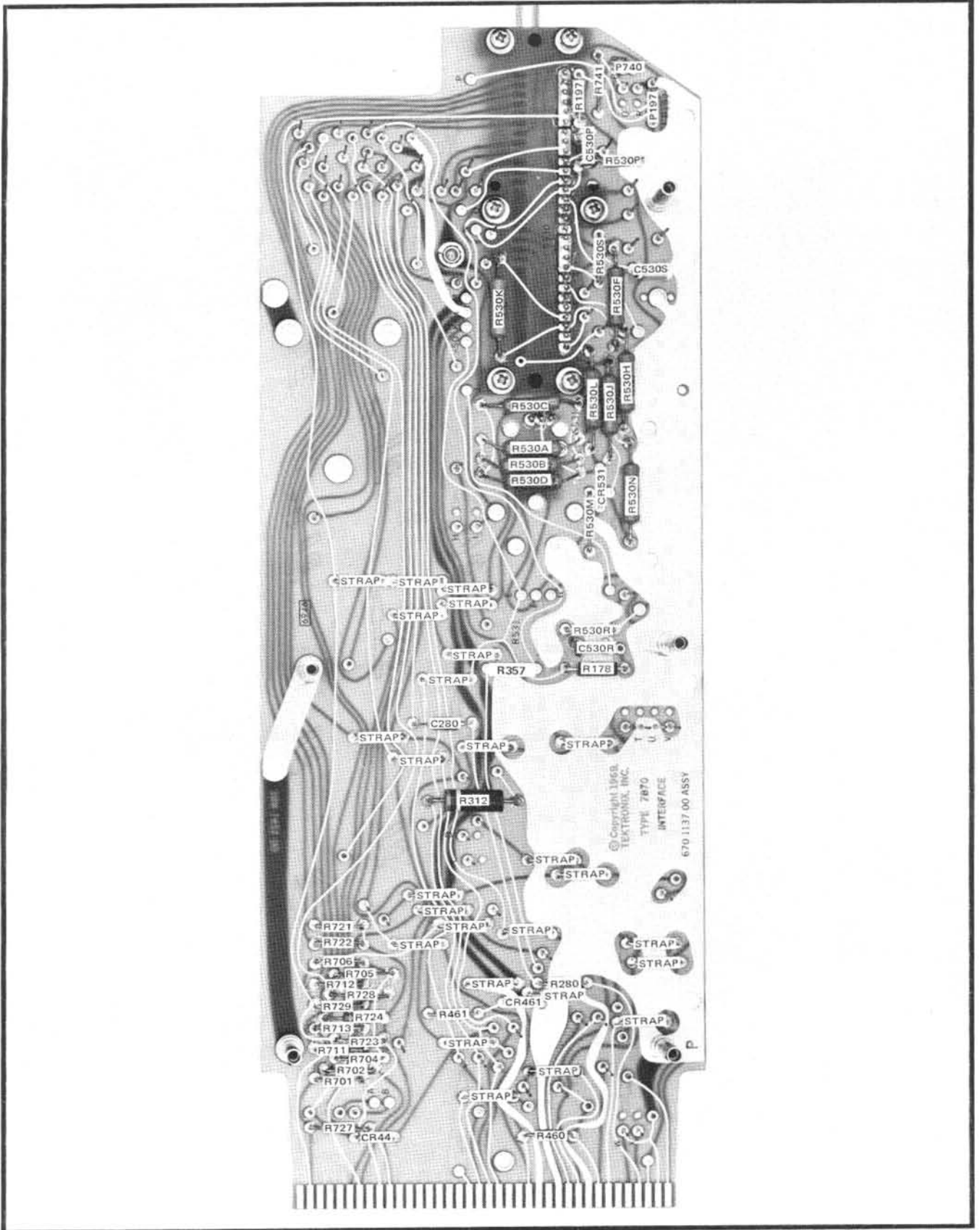
Fig. 4-6. Interface board showing location of components.
