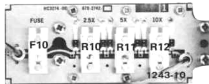
A2 7A19 Amplifier board Attenuator circuit board assembly above SN B030000.
