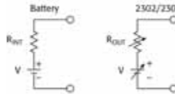
Simplified schematic of a battery and the 2302/2306.
