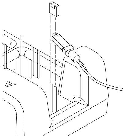
After you are finished with this probe, be sure to replace the small jumper.
