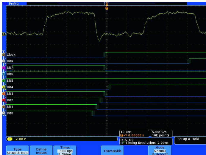
Multichannel setup and hold triggering highlighting multiple violations (MSO4000).
