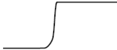
Signal with a short ground lead
