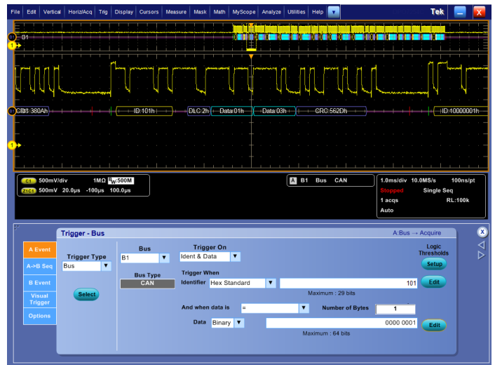
Triggering on a specific ID and data value on the CAN bus.
