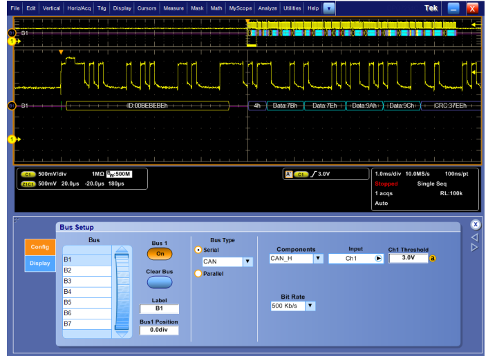
CAN bus setup, showing assignment of source, threshold, and bit rate.
