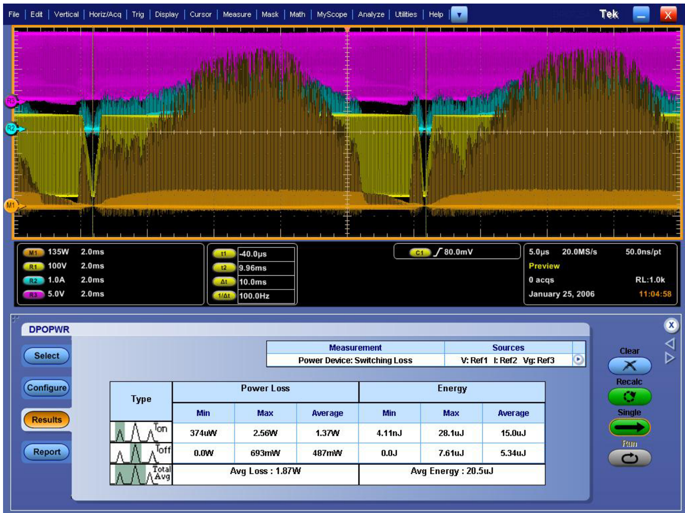
Figure 21: Switching Loss results
