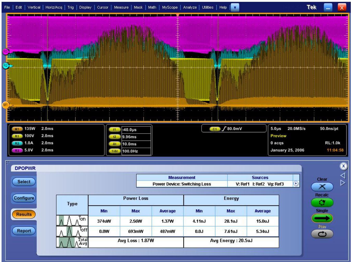
Figure 98: Switching Loss Results
