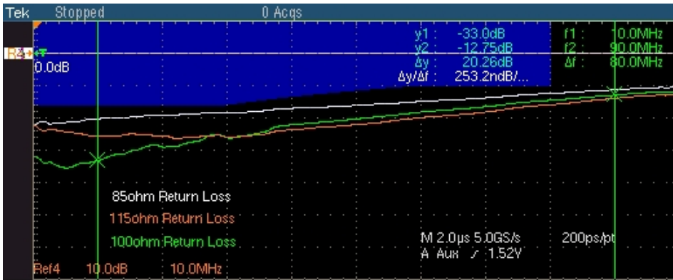
Figure 9-18: Waveform for 100BASE-TX Return Loss Transmitter
