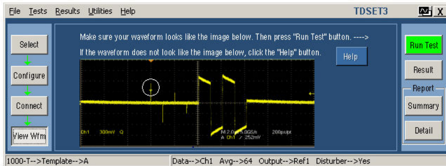
Figure 11-1: 1000BASE-T View Waveform for Template, Peak Volt, and Droop with disturbing signal
