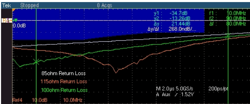
Figure 9-19: Waveform for 100BASE-TX Return Loss Receiver
