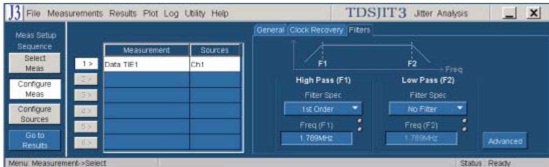
Figure 98: Configuring filters for a 1.5 Gbps SAS device
