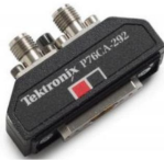
P76CA-292 33 GHz Bandwidth Coaxial Adapter with 2.92 mm (Female) connectors. This adapter is calibrated at the input connectors and is ideal for use with off the shelf or custom cables. Low skew cable pairs should be used to preserve full bandwidth performance.
