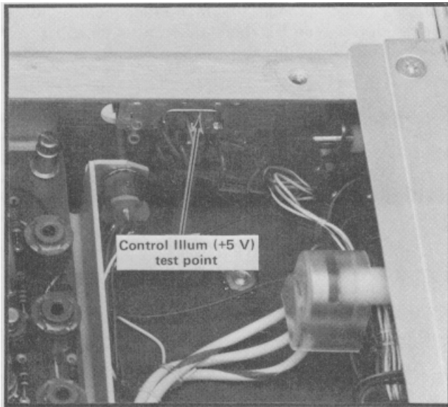
Fig. 5-2. Location of Control Illum. (+5 V) test point (bottom of instrument).
