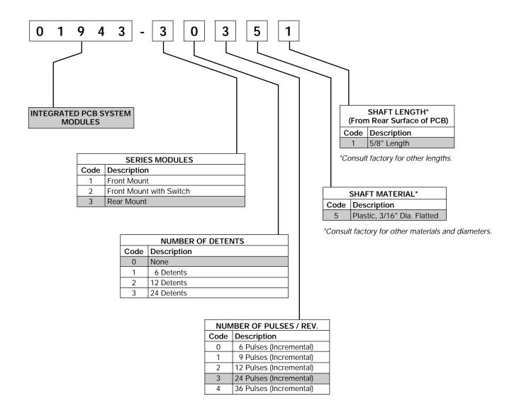
NOTE: This chart illustrates the numbering system for the module level only.
