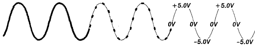
Figure 2-3: Acquisition: Input Analog Signal, Sample, and Digitize
