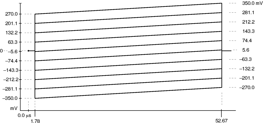
Figure 17: Shallow Ramp (10 possible amplitudes), B-Y and R-Y
