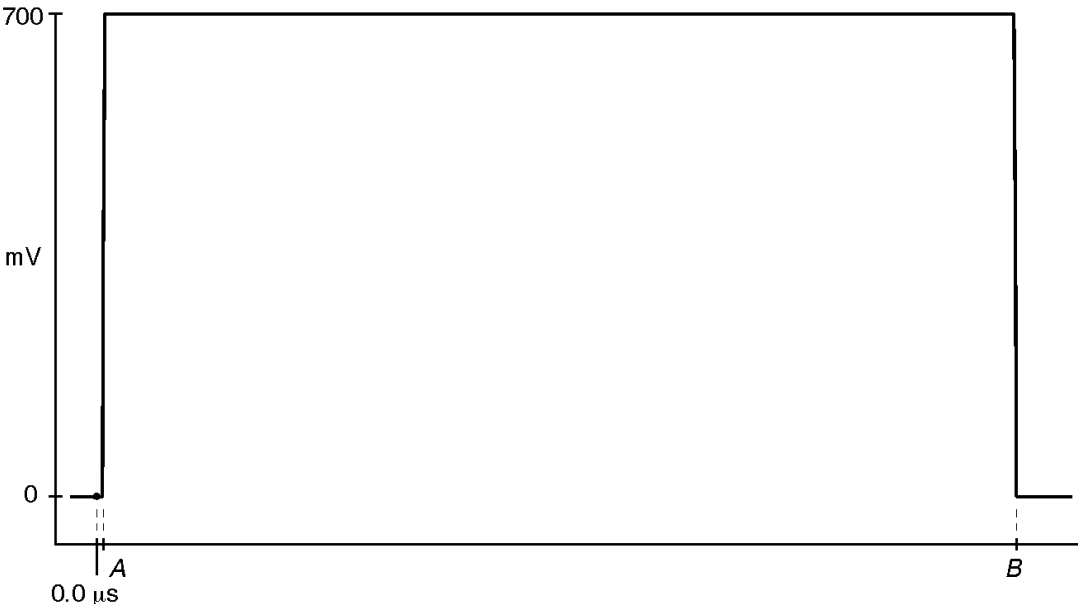
Figure 31: Active Picture Markers, vertical limits, Y channel only
