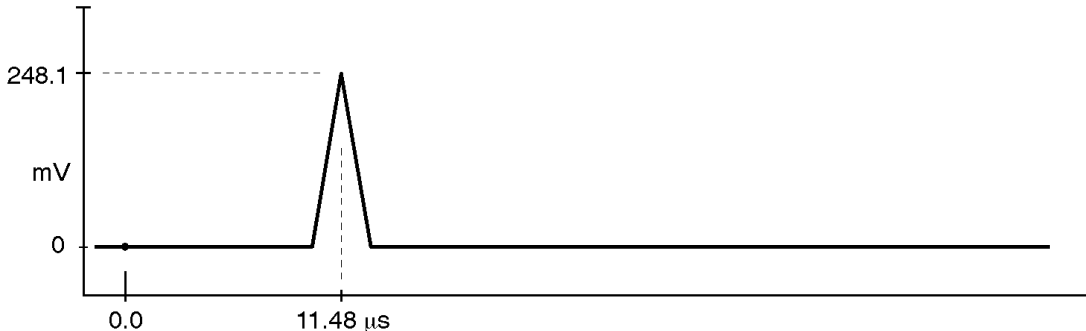
Figure 23: 525 Line Mod Pulse and Bar, R-Y
