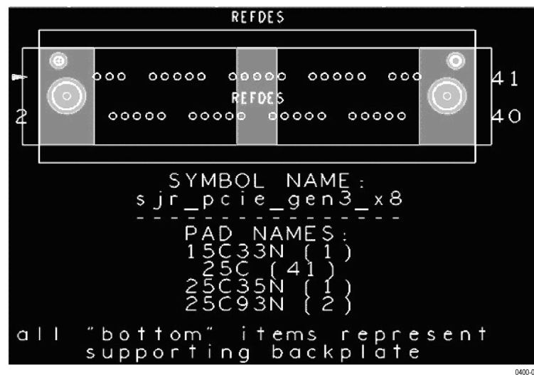
Figure 57: P67SA16 x8 midbus probe CAD symbol
