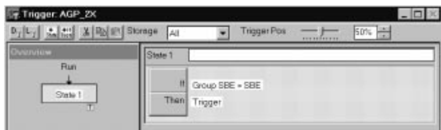
Figure 2–11: Trigger setup for any SBE cycle in the Status channel group
