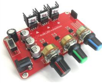
RGB LED Brightness Controller with 555 Timer
