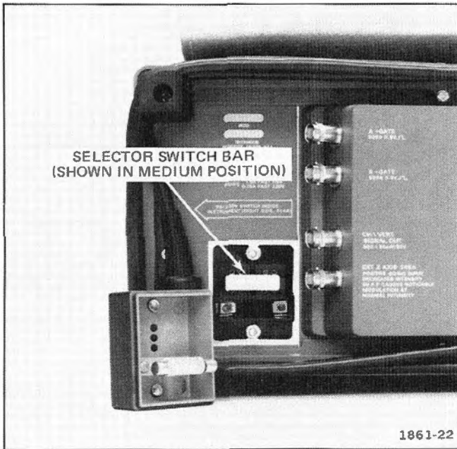
Fig. 2-1. Power supply regulating range selector.
