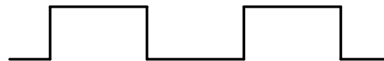
(d) Resultant Waveform Seen at the Output of the AM 503A—a Combination of (b) and (c)
