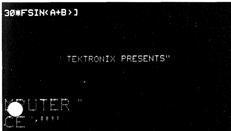
Fig. 1. The 84-character refreshed memory shown below, allows text to be quickly and easily corrected and edited before being sent to the computer.
