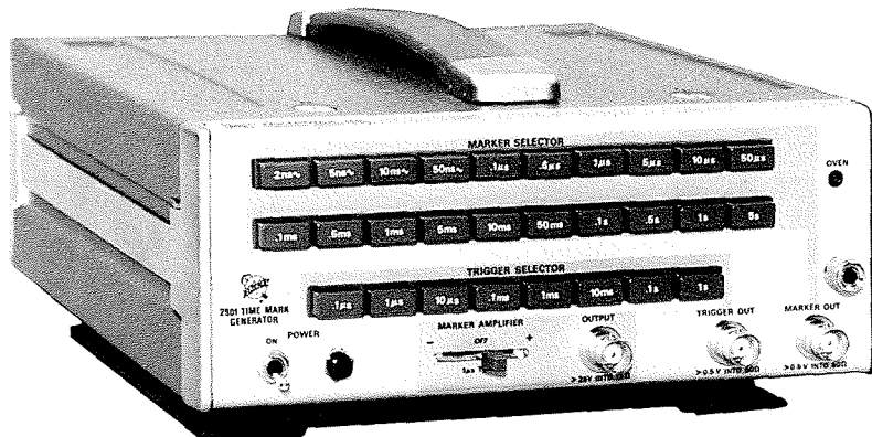
This precision time or period source produces sixteen timing pulses by digital countdown. Maximum countdown ratio is 5 \times 10^{11} from an internal precision source. The 2901 will also accurately countdown external signals.
