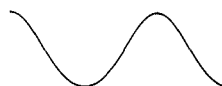
A sinewave with approximately 6% second harmonic content to provide piston volume as a function of crankshaft rotation ( r/l = 1/4 ).
