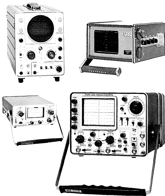
DC-powered Oscilloscopes manufactured by Tektronix which use NiCd sealed cells. Pictured are the Type 321A (DC 6-MHz), Type 410 Physiological Monitor, Type 323 (DC 4-MHz) and Type 422 Mod 125B (DC 15-MHz).
