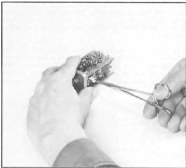
Fig. 4-2. Removal or replacement of sampling bridge diodes.
