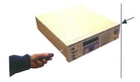
To allow the top cover to be slid back the two side screws must be removed (note the front panel has 3 fixings at the bottom of the panel – these only need to be removed if the front panel needs to be dropped down or removed).
