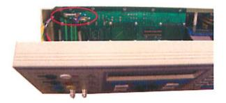
To allow the front panel to be dropped down for access to the front panel fuses, remove the screws from both sides of the front panel assembly, shown above. The fuses are located in PCB mounted fuse holders as shown above, right. Replace these fuses with the same type and rating – 2A Ultra Rapid
