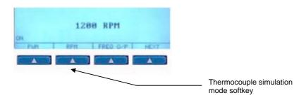
TIP: If the RPM menu item is not displayed, press the NEXT softkey to go to the next menu level.
