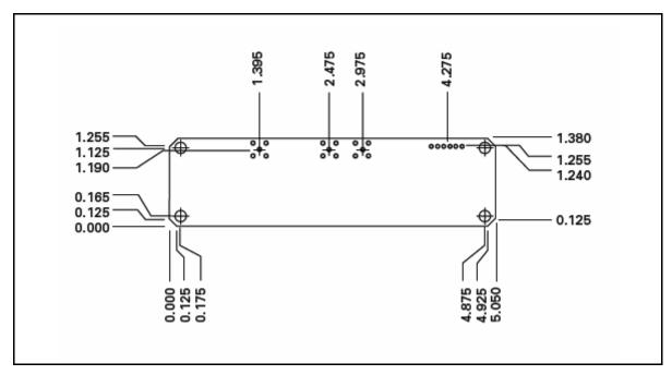
The base mounting screw holes (4) accommodates #6/32 x 3/8 machine screws. When mounting the Mini-T onto a plate for permanent mounting, take into consideration the length of the screw and the thickness of the plate so that the screws do not protrude into the Mini-T and potentially damage electronics.
