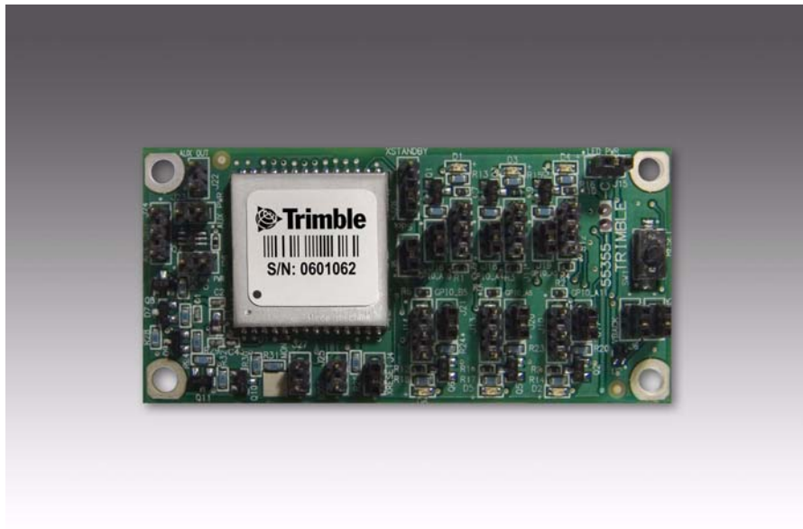
Figure 10.1 Copernicus Reference Board, Frontside
