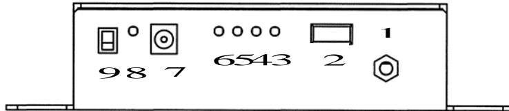
Figure 11.4 Front side of the Interface Unit
