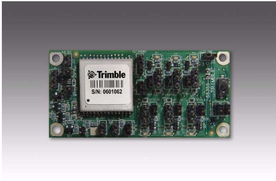
Figure 10.1 Copernicus Reference Board, Frontside
