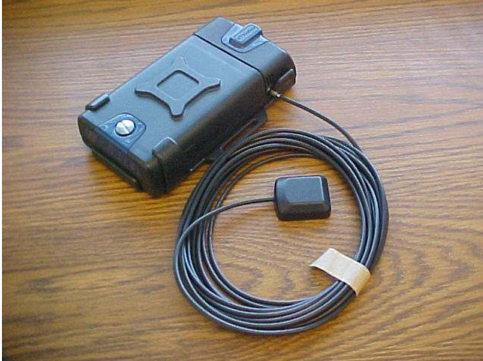
Figure 10. External GPS Antenna Connected to TrimTrac 1.5
