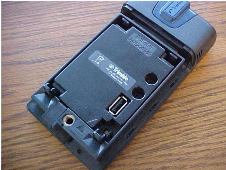
Figure 22. Properly Inserted Provisioning Module.
