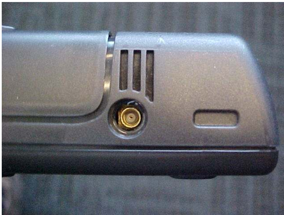
Figure 9. External GPS Antenna RF Connector.
