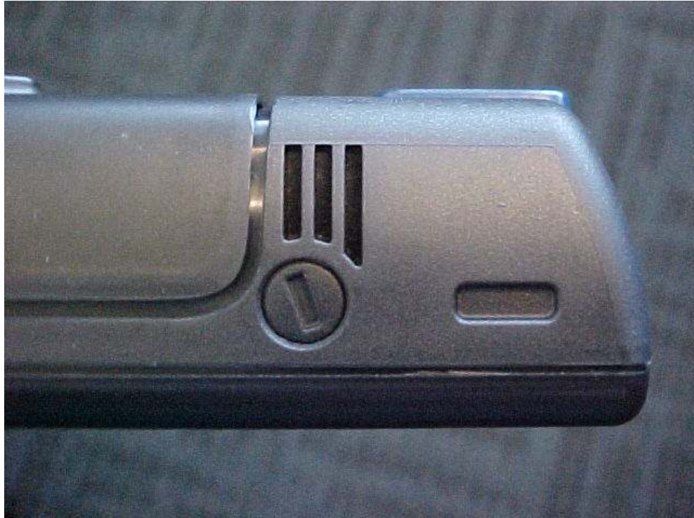
Figure 8. External GPS Antenna RF Connector Plug.
