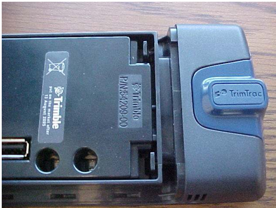
Figure 23. Provisioning Module Improperly Inserted. Upper Tab not Latched Properly.
