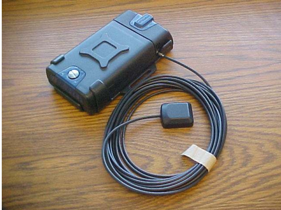
Figure 1. TrimTrac 1.5 Shown with Optional External GPS Antenna and Quick Release Bracket.
