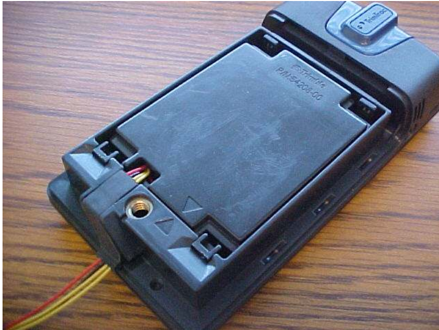
Figure 4. Vehicle Adapter Module inserted into a TrimTrac 1.5
