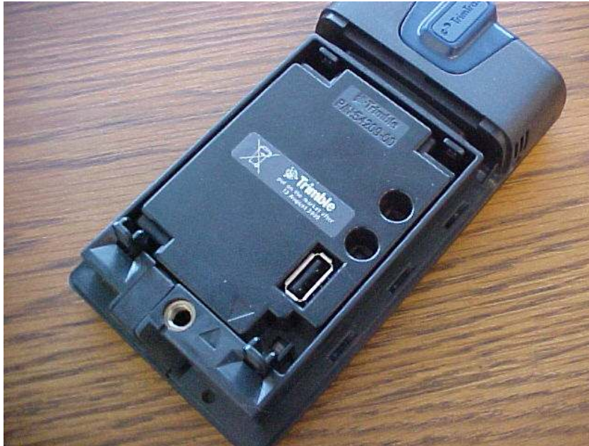
Figure 3. Provisioning Module inserted into a TrimTrac 1.5
