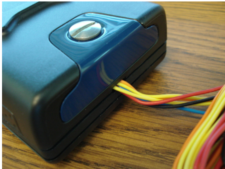
Figure 16. Cover in place with Wires Properly Routed
