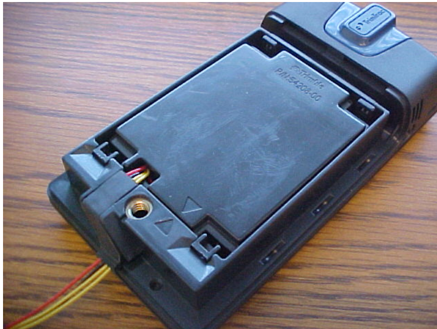
Figure 4. Vehicle Adapter Module inserted into a TrimTrac Pro
