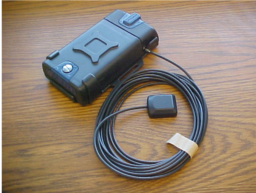
Figure 19. External GPS Antenna Connected to TrimTrac Pro
