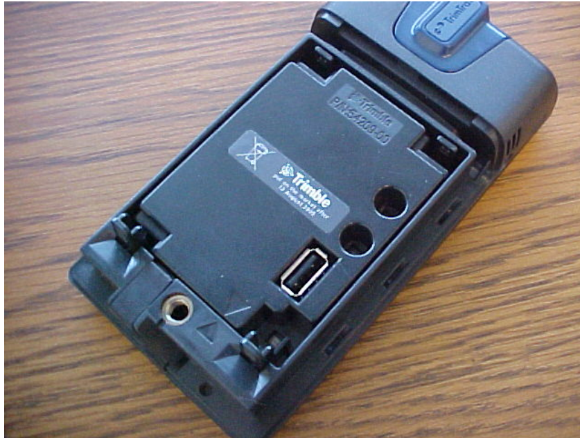
Figure 3. Provisioning Module inserted into a TrimTrac Pro
