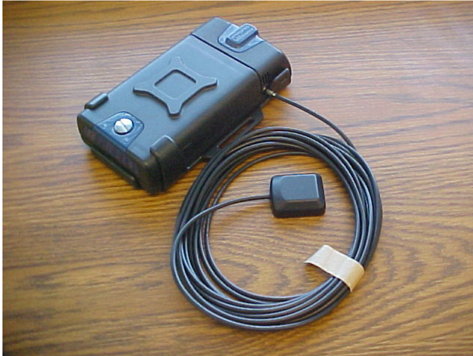
Figure 1. TrimTrac Pro Shown with Optional External GPS Antenna and Quick Release Bracket.
