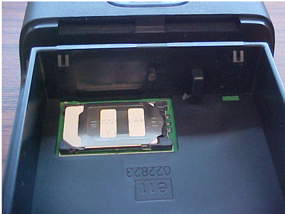
Figure 30. Properly Latched SIM Card Holder.
