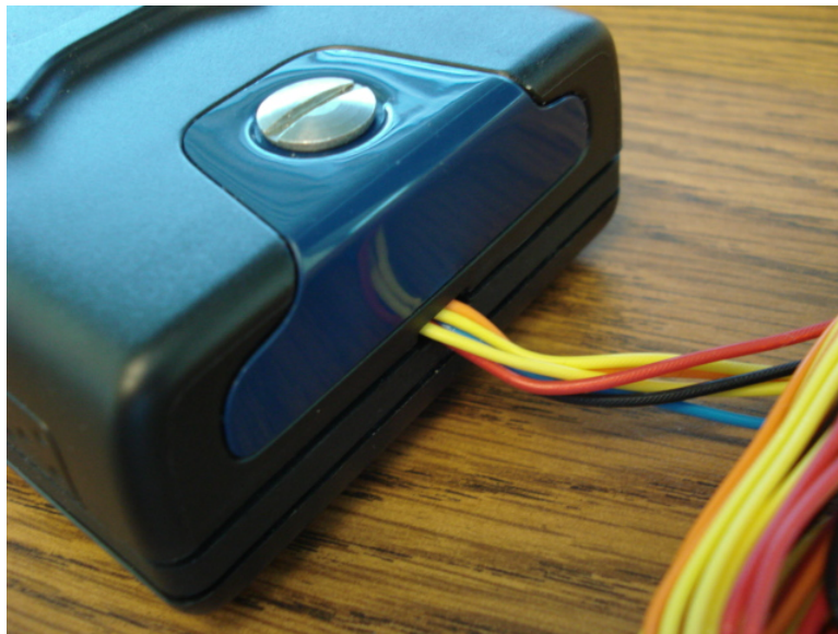
Figure 16. Cover in place with Wires Properly Routed
