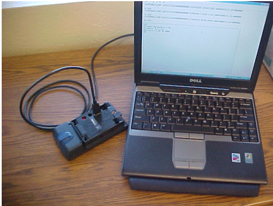
Figure 33. TrimTrac Pro Connected to PC via Provisioning Module and USB A-to-A Cable.
