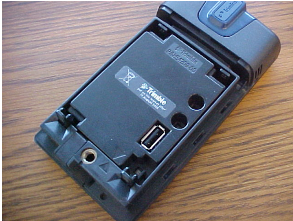
Figure 31. Properly Inserted Provisioning Module.
