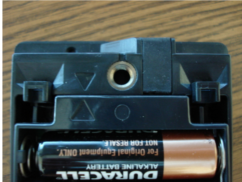
Figure 11. Align Arrows on base and module.
