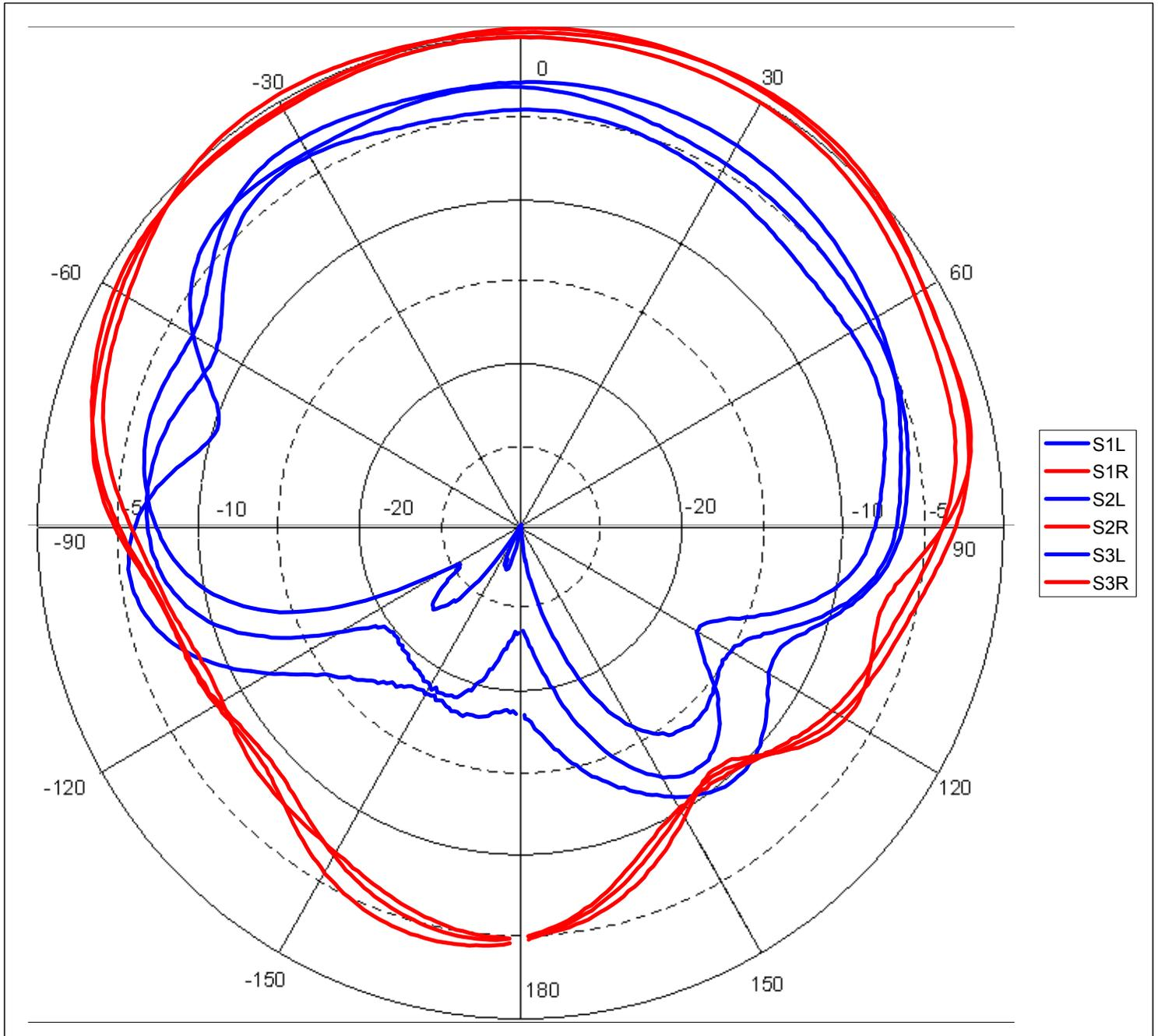
Small patch antenna mounted on a 105mm by 44mm plate 1.3mm thick
