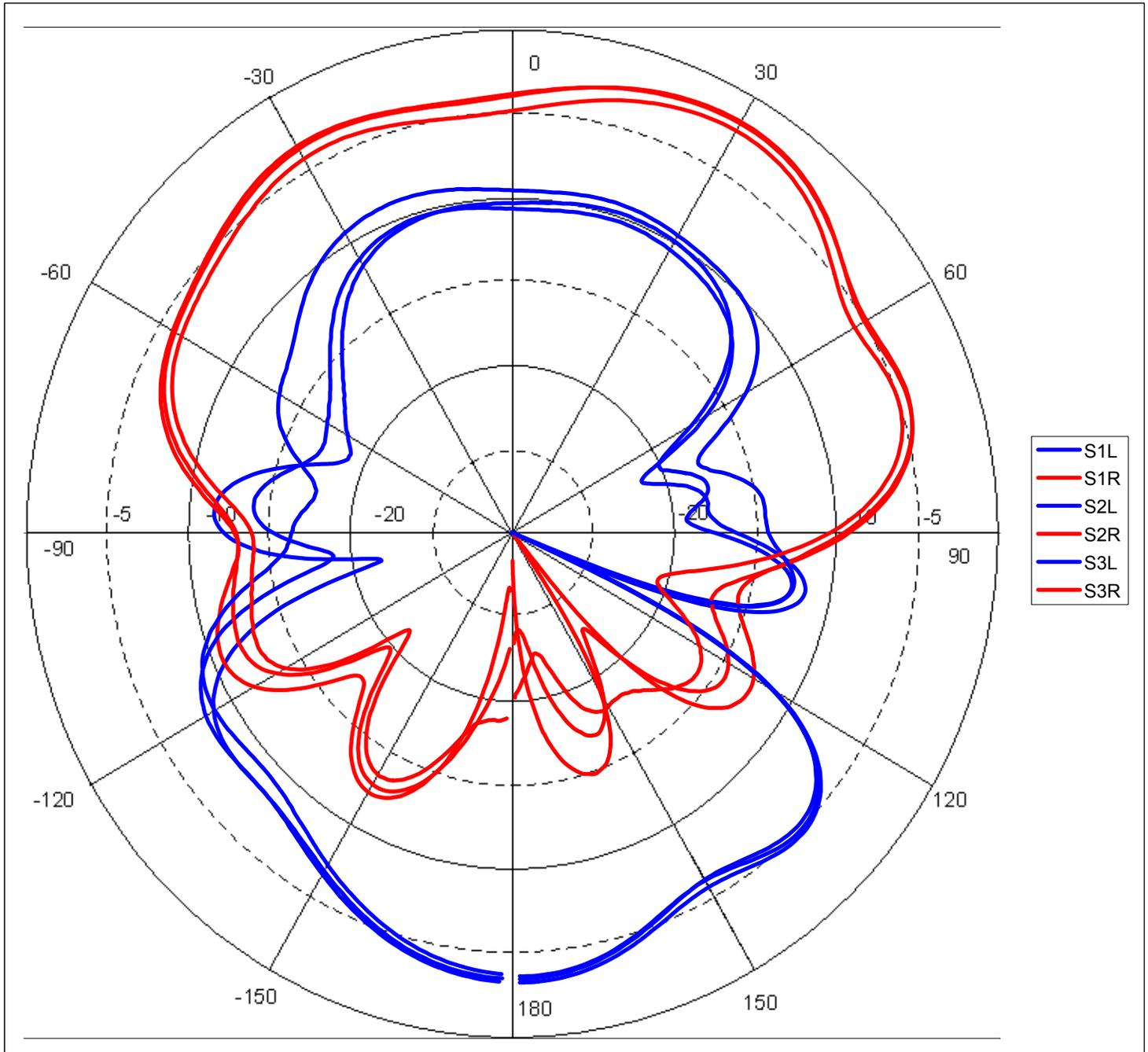
Small patch antenna mounted on a 40mm square plate 6mm thick
