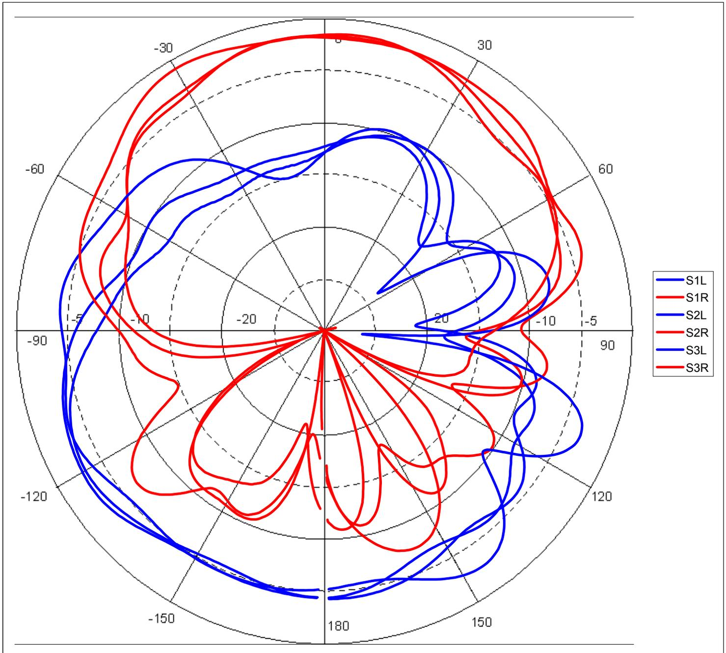
Small patch antenna mounted on a 26mm square plate 7mm thick
