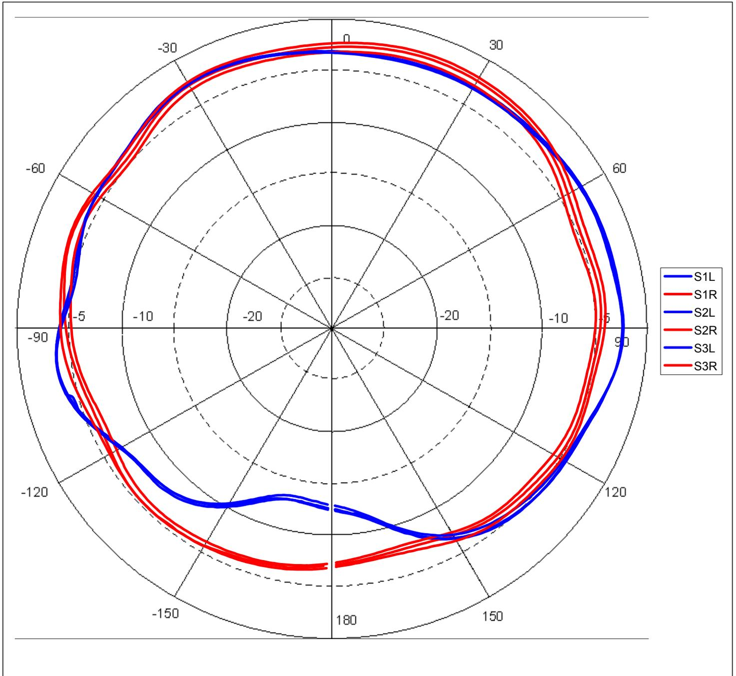
Small patch antenna mounted top middle edge of a 200mm by 150mm rectangular plate 20mm thick
