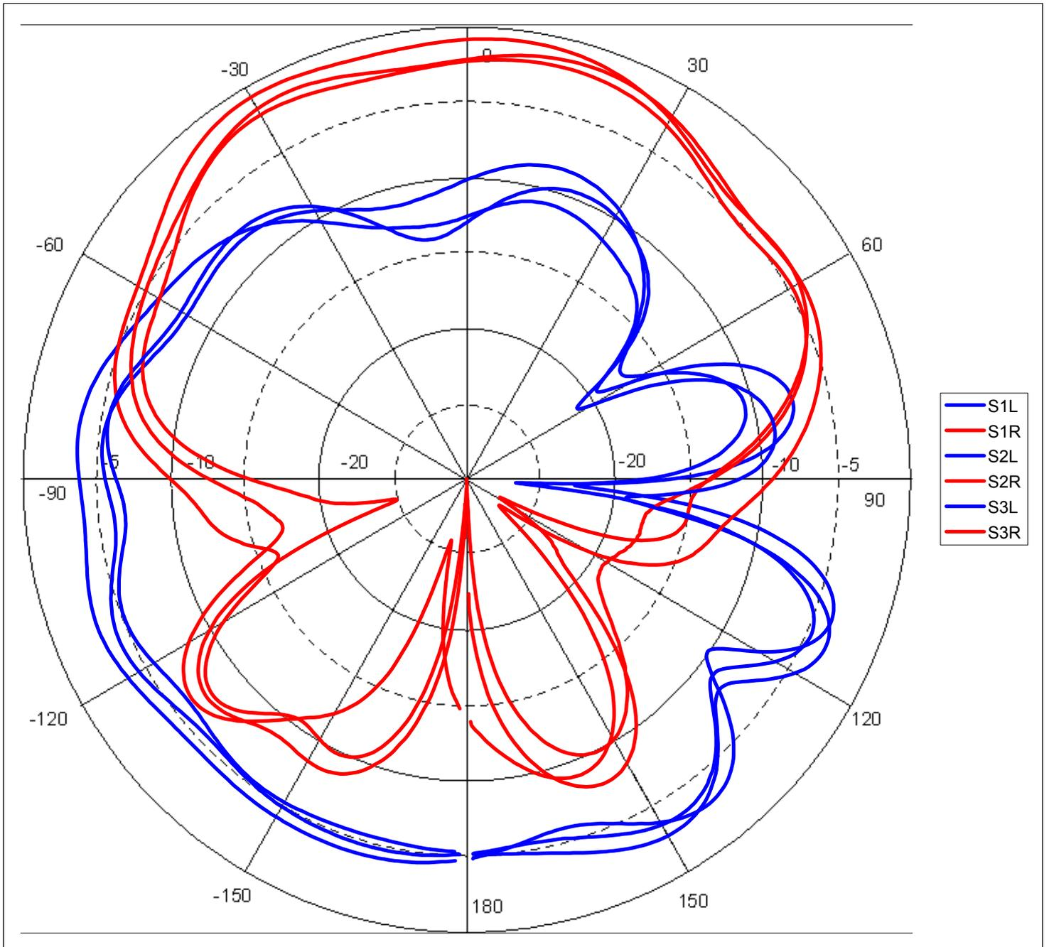
Small patch antenna mounted on a 26mm square plate 17mm thick
