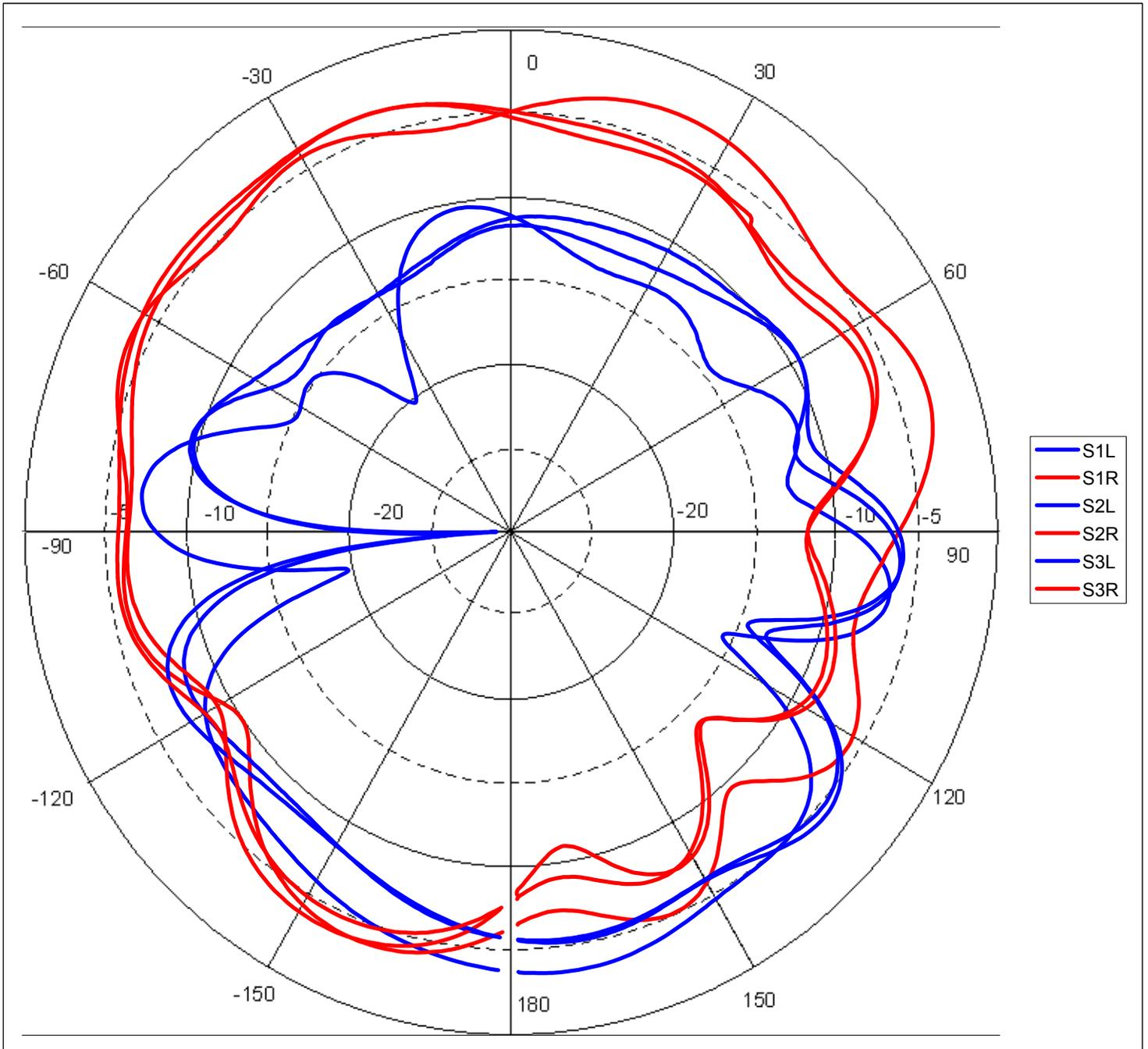
Small patch antenna no ground plane
