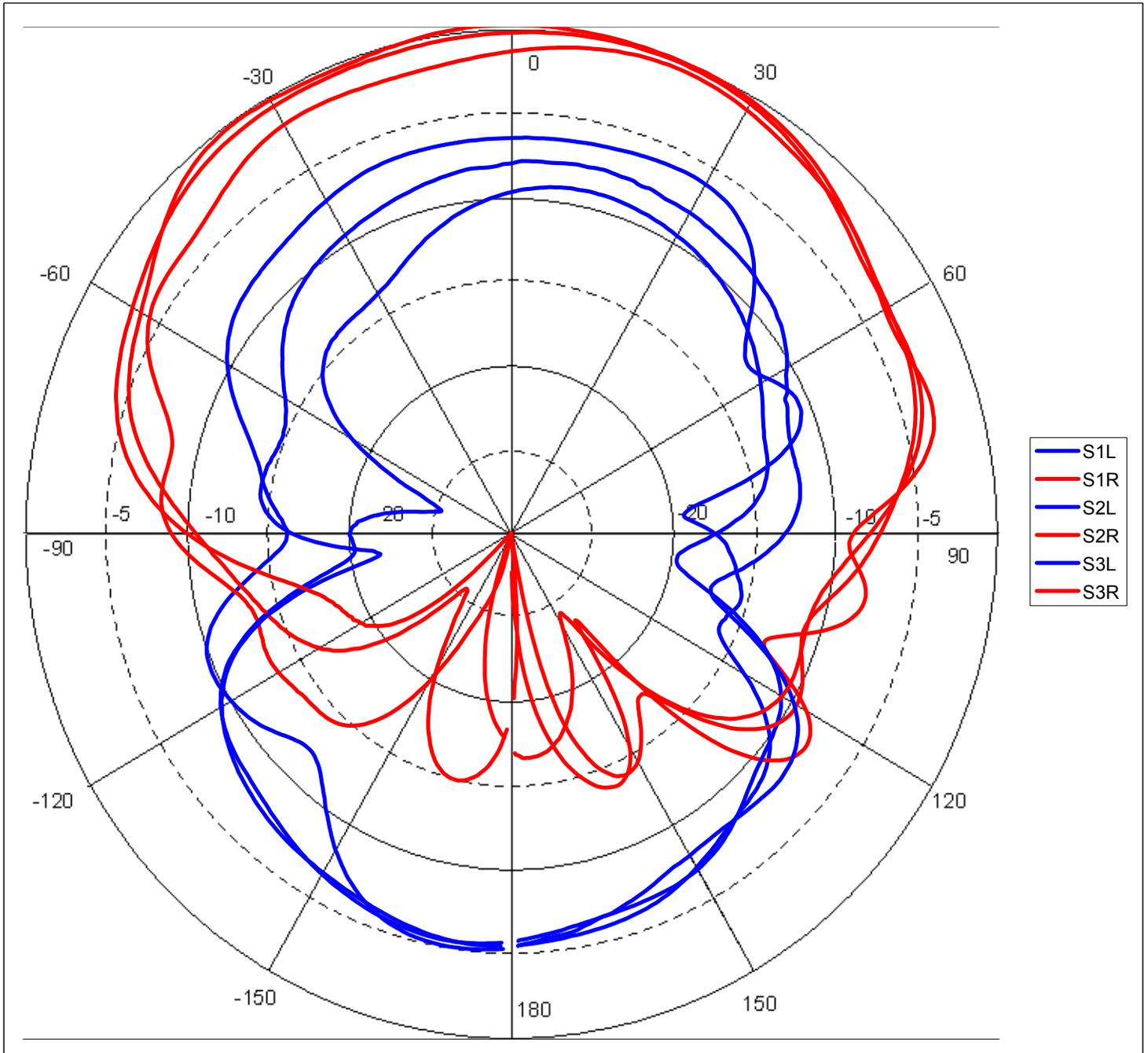
Small patch antenna mounted on a 60mm round plate 12mm thick
