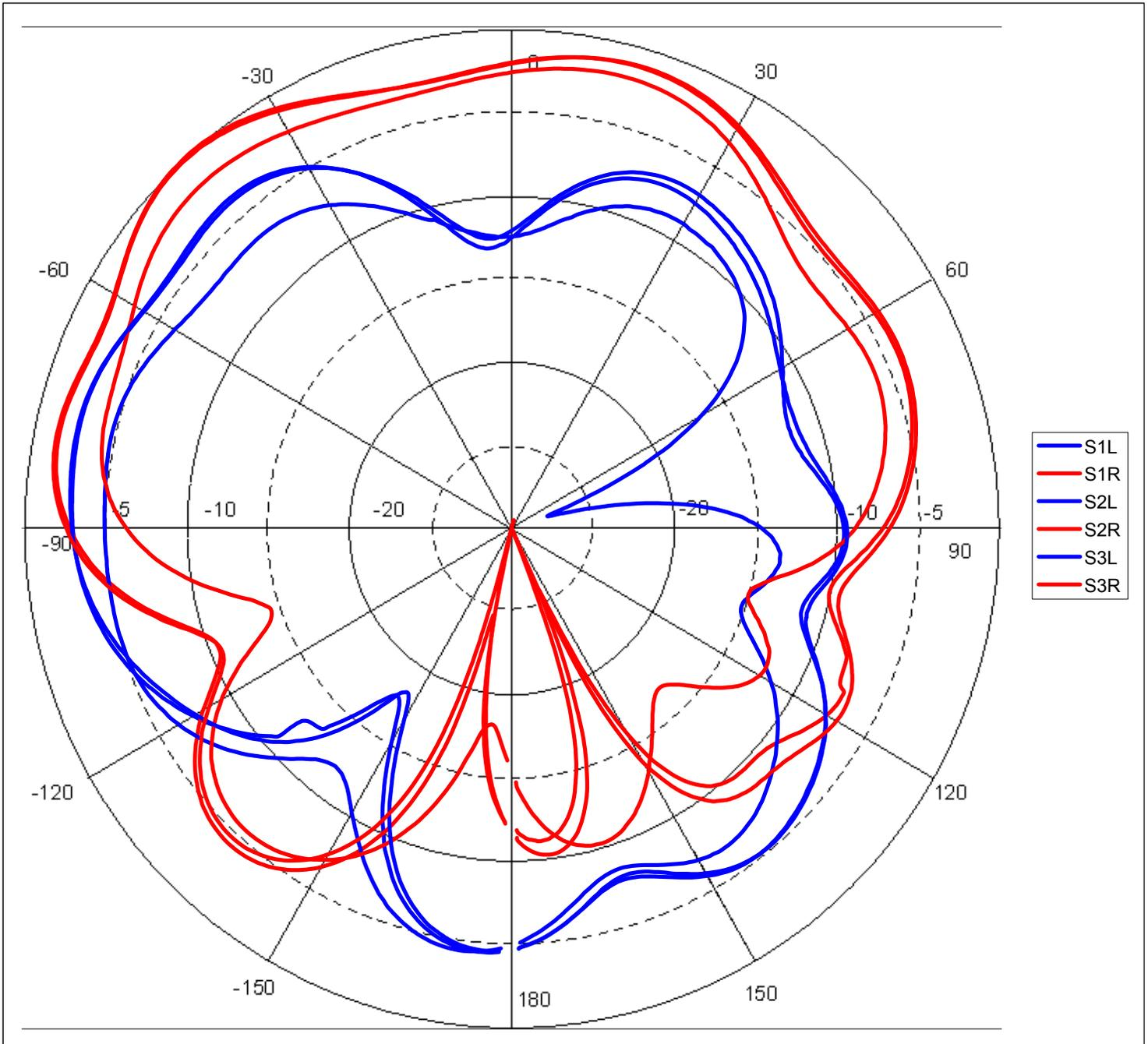
Small patch antenna mounted top corner edge of a 200mm by 150mm rectangular plate 20mm thick
