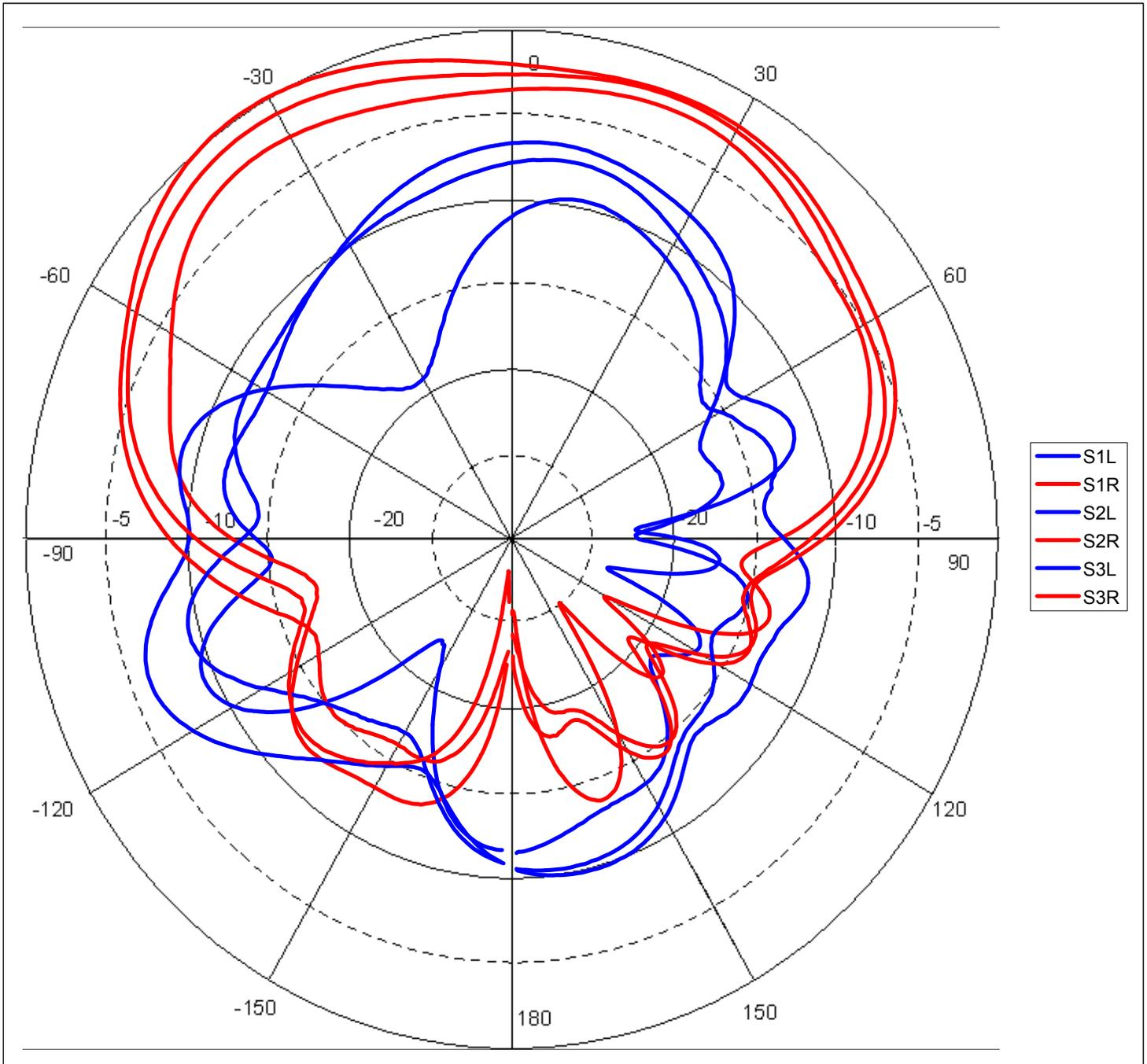
Small patch antenna mounted top corner of a 200mm by 150mm rectangular plate 20mm thick
